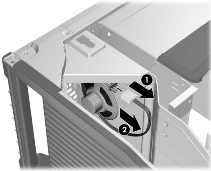
Figure 5-12 Removing the speaker
