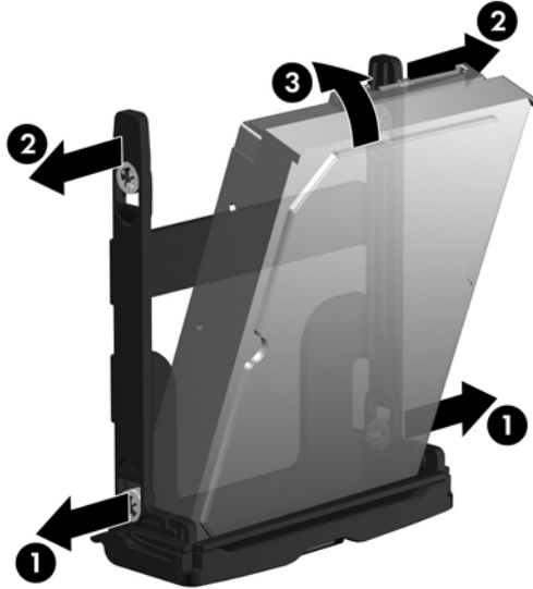
Figure 5-43 Installing the drive in the carrier
