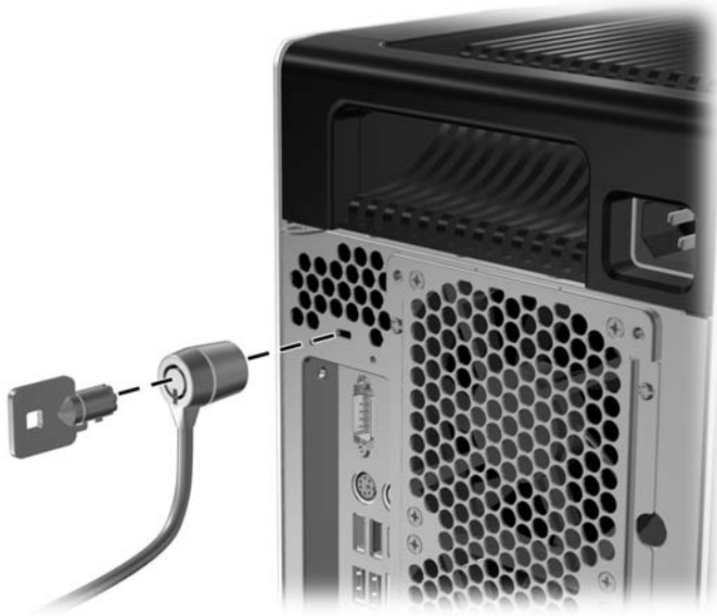
Figure 5-2 Removing the cable lock
