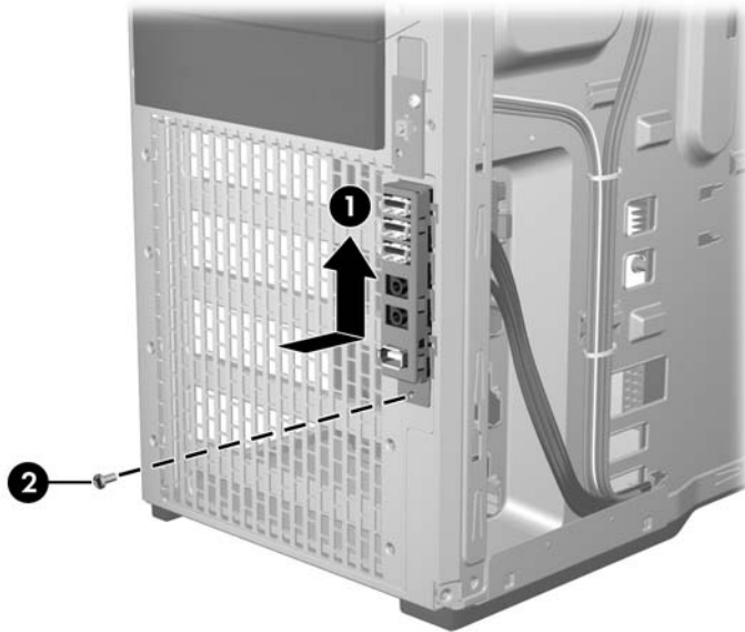
Figure 5-18 Installing the front panel I/O cable assembly
