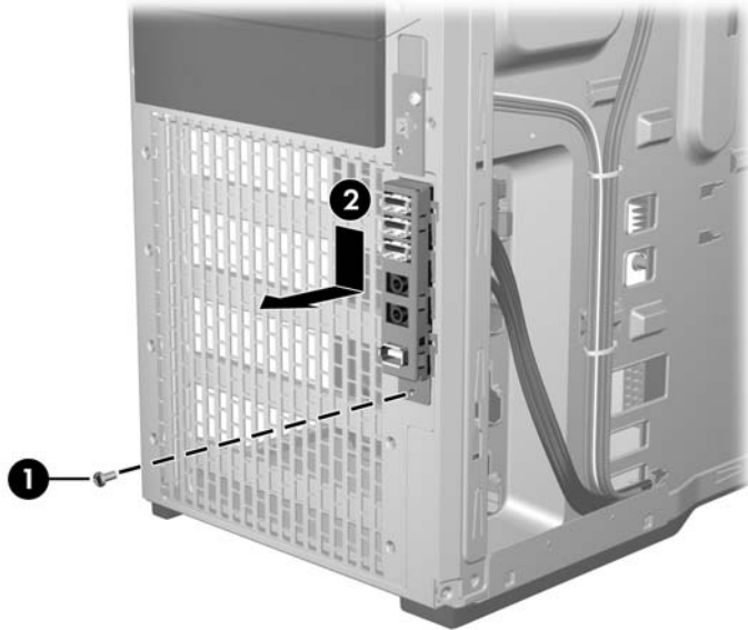
Figure 5-17 Removing the front panel I/O cable assembly
