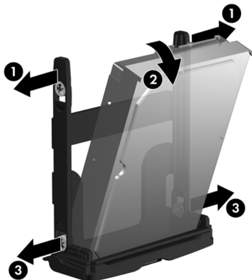
Figure 5-40 Removing the drive from the carrier
