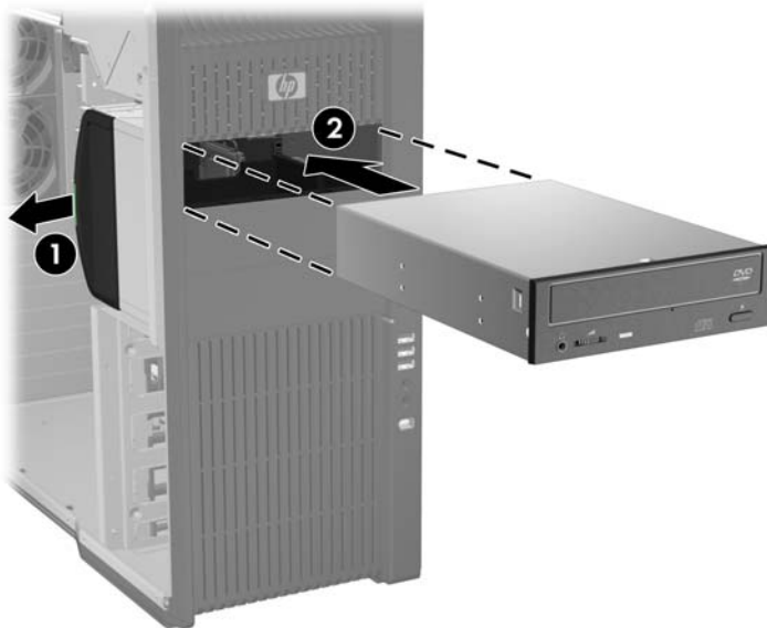
Figure 5-26 Installing the optical disk drive
