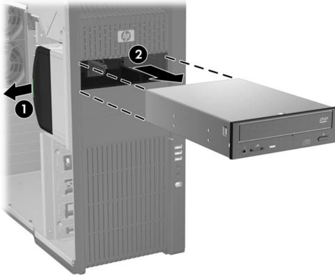
Figure 5-25 Removing the optical disk drive
