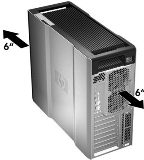
Figure 1-5 Proper workstation ventilation
