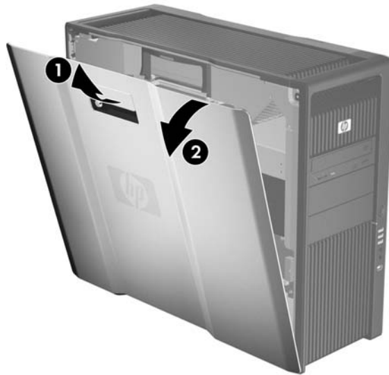
Figure 5-3 Removing the side access panel
